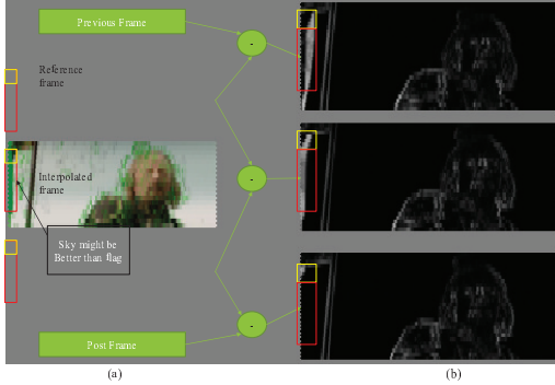
Fig. 3. (a) Classifying foreground versus background in a hole area, (b) difference map example of adjacent frames from [2]
